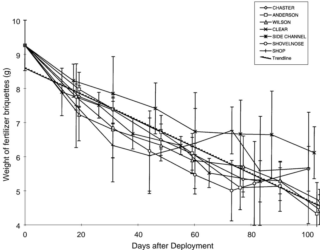
Figure 1. The rate of dissolution of the fertilizer briquettes is demonstrated; the reduction of weight over time is approximately 0.5% per day.
