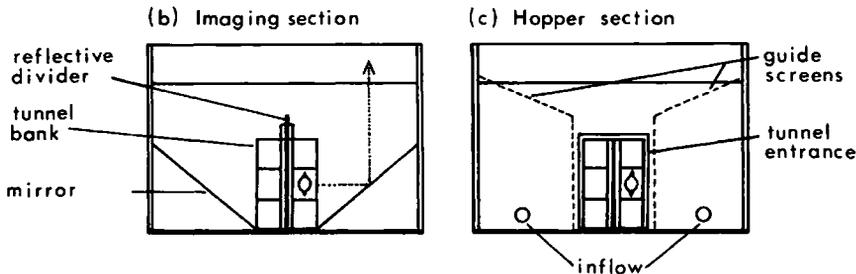
FIGURE 1.—Diagrams of the fish inventory system used to videotape coho salmon smolts at the Keogh River. (a) A cut-away side view of the entire experimental apparatus. (b) A cross section of the imaging section. (c) A cross section of the hopper section.
